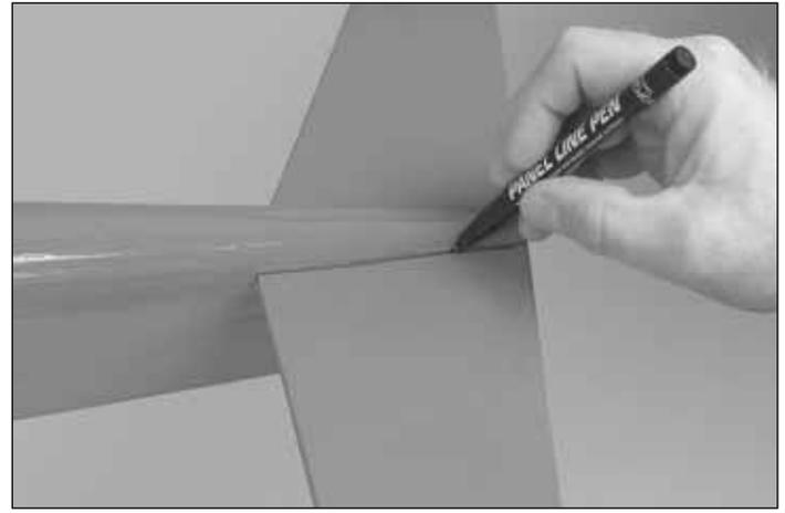
❑ 6. Use a fine-point felt-tip pen to mark the outline of the fuselage onto the bottom and top of the stab.
