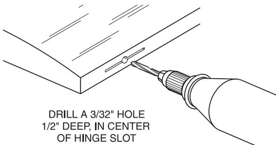
DRILL A 3/32" HOLE 1/2" DEEP, IN CENTER OF HINGE SLOT
