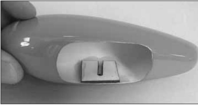
❑ ❑ 5. Use sandpaper to roughen the inside of the wheel pant in the area around the mounting slot. Clean the area with denatured alcohol. Trial fit the plywood wheel pant mounting plate inside the wheel pant. The top edge of the mounting plate may need to be rounded to match the curve of the wheel pant. Once satisfied with the fit, use epoxy to glue the mounting plate in the wheel pant.
