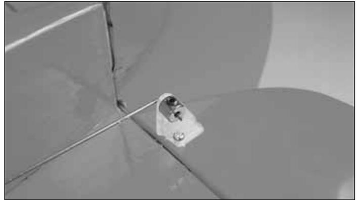
❑ 4. Connect the pushrod wire to the control horn with a 1.7mm wheel collar and 2.5mm set screw.
