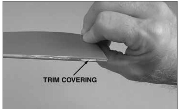
❑ 13. Trim the covering from the elevator joiner wire slot in the leading edge of both elevator halves.
