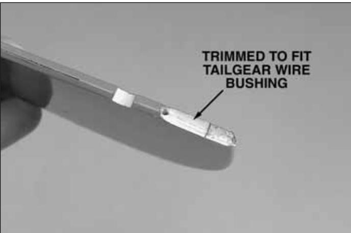
❑ 19. Drill a 3/32" [2.4mm] hole into the leading edge of the rudder at the mark. Cut a slot in the leading edge of the rudder to clear the tail gear wire bushing.
