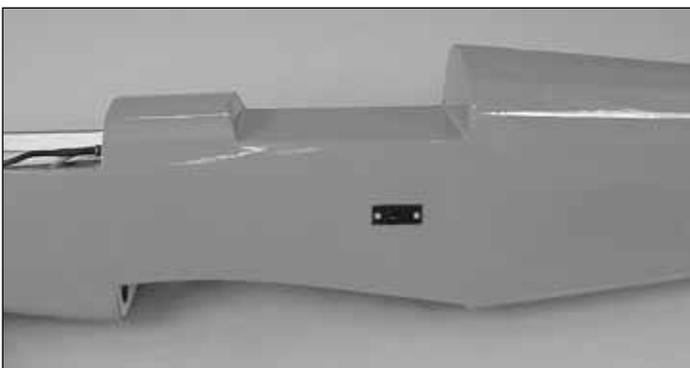
❑ 4. Plug the ESC into the throttle channel in the receiver. Connect the red and black "bullet" connectors from the ESC to the connectors from the motor. Remove the cover from the on/off switch. Mount the on/off switch on the fuselage just behind the servo tray.
