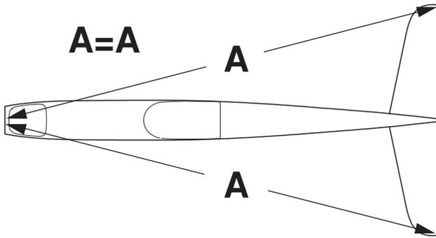
❑ 4. Fold a piece of masking tape over the other end of the string and draw an arrow on it. With the stab centered on the fuselage, slide the tape along the string and align the arrow with one tip of the stab. Swing the string over to the same position at the other end of the stab. If the arrow doesn't align with the tip, adjust the stab and the arrow slightly and check both tips again. Adjust the stab until the stabilizer tips and the trailing edge are centered.
