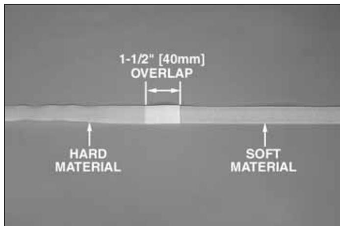
5. To make the battery strap, overlap the two pieces of hook-and-loop material as shown.
