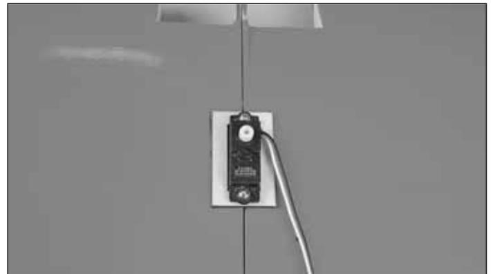
❑ 8. Mount the aileron servo in the wing. Use CA to harden the threads. Plug a 6" [150mm] aileron servo extension into the receiver. Connect the aileron servo to the servo extension and switch on the transmitter and ESC. Center the aileron servo trim.
