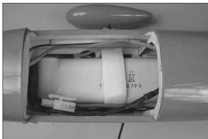
6. Insert the hook-and-loop strap through the slot in one side of the battery tray and bring it out the slot in the other side of the tray. Adjust it so that the overlap is under the tray. Install the battery in the battery compartment and secure it with the hook-and-loop strap. Trim off the excess hook-and-loop material.
