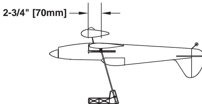
2. With the wing attached to the fuselage, all parts of the model installed (ready to fly) and the motor battery installed, place the model upside-down on a Great Planes CG Machine, or lift it upside down at the balance point you marked.
