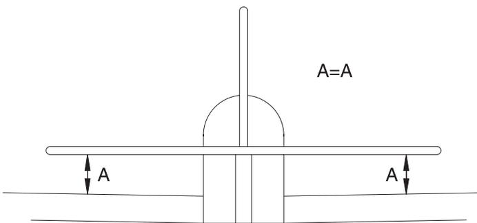
❑ 5. View the stab from approximately 10' [3m] behind the plane. Check that the stab is parallel with the wing. If it is not, lightly sand the stab saddle until the stab is parallel with the wing.
