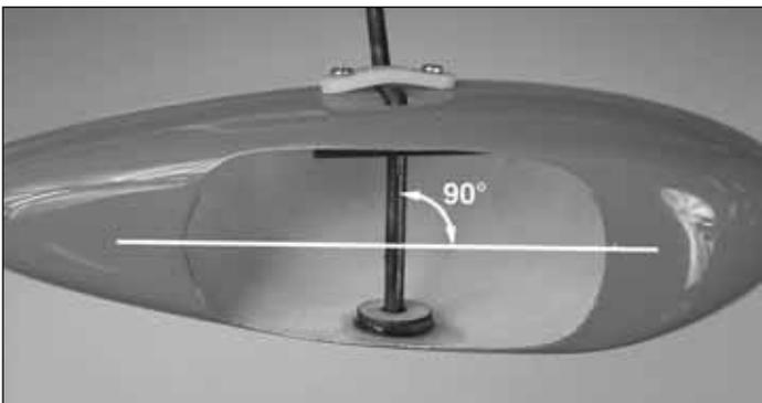
❑ ❑ 7. Remove one of the screws from the landing gear strap and slide a round plywood wheel pant retainer onto the landing gear. Re-attach the landing gear strap. Align the axle of the landing gear so that it is perpendicular to the centerline of the wheel pant. Apply a thin coat of oil or petroleum jelly on the axle to prevent the epoxy from adhering. Roughen the inside of the wheel pant and glue the wheel pant retainer to the wheel pant with epoxy.
