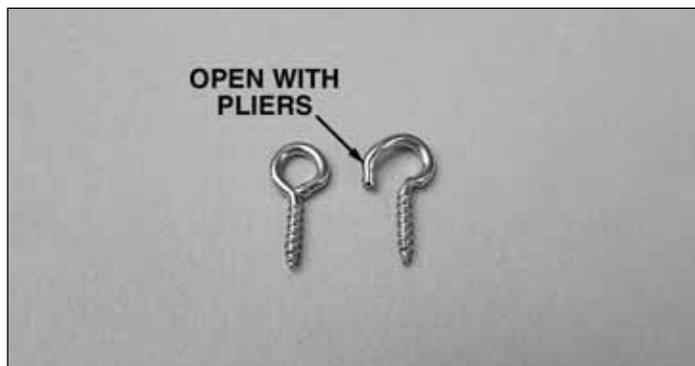
1. Use a needle-nose pliers to open the two eye hooks.
