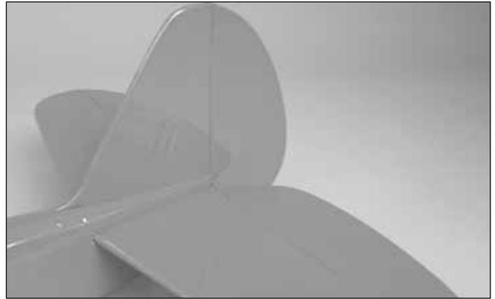
❑ 20. Once satisfied with the fit of the tail gear wire in the rudder, apply epoxy in the tail gear wire hole in the leading edge of the rudder. Join the rudder to the fin using two CA hinges. Before the epoxy cures, use thin CA to glue the CA hinges in the rudder and fin following the same procedure used for the ailerons.
