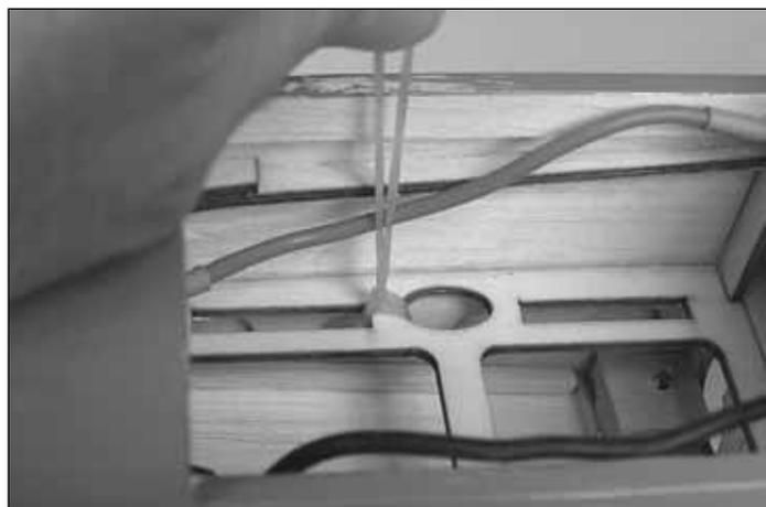
3. Tie two rubber bands, one on each side of the battery tray. Making a hook from a paper clip will help in pulling the rubber band through the tray.
