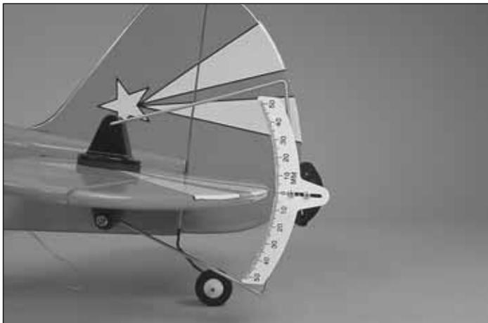
Use a Great Planes AccuThrow (or a ruler) to accurately measure and set the control throw of each control surface as indicated in the chart that follows. If your radio does not have dual rates, we recommend setting the throws at the low rate setting. **NOTE:** The throws are measured at the **widest part** of the elevators, rudder and ailerons.
