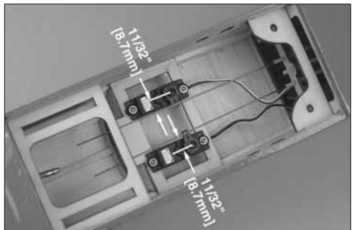
❑ 1. Install servo arms on the rudder and elevator servos. The pushrod mounting holes should be approximately 1 1/32" [8.7mm] from the center of the servo arm. Install the rudder and elevator servos in the servo tray, aligning the hole in the servo arm with the pushrod wire. Use the hardware included with the servos to mount the servos to the tray. After installing the servo mounting screws, remove them, apply a drop of CA to each hole to harden the threads, then reinstall the screws.
