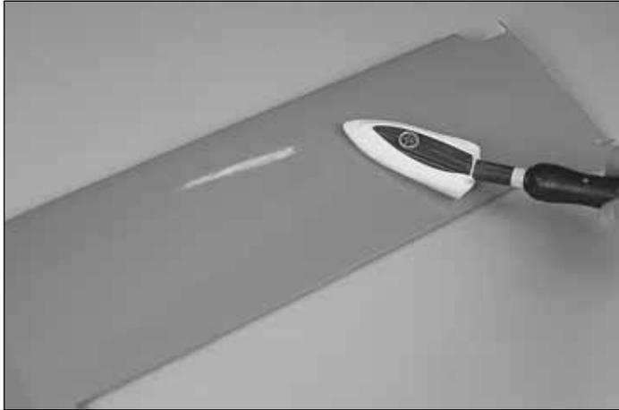
2. Remove the masking tape and separate the ailerons from the wing, the rudder from the fin and the elevator from the stabilizer. If necessary, use a covering iron set on medium/high to tighten the covering. Apply pressure over sheeted areas to **thoroughly** bond the covering to the wood.
