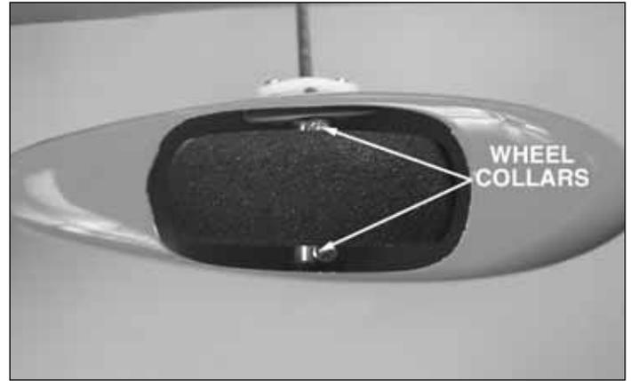
❑ ❑ 8. Install a 3x4mm machine screw in two 3mm wheel collars. Remove one of the screws from the landing gear strap and install on the landing gear a wheel collar, wheel and a second wheel collar. Insert the landing gear in the wheel pant retainer and reinstall the landing gear strap. Tighten the 3x4mm machine screws in the two wheel collars. Make sure that the wheel rotates freely.
