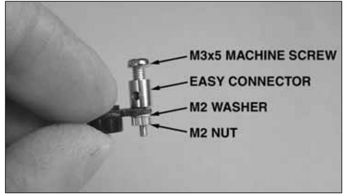
❑ 5. Install the two pushrod connectors on the rudder and elevator servo horns by first inserting the connector through the horn, then install a 2mm washer and an 2mm nut on the connector. Apply a drop of threadlock to the 3x5mm machine screw and install in the top of the pushrod connector.
