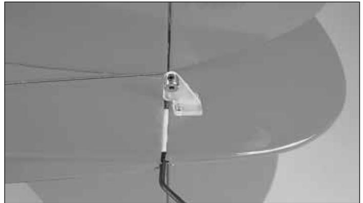
❑ 5. Install the rudder control horn following the same procedure. Make sure that the control horn does not interfere with the elevator.
