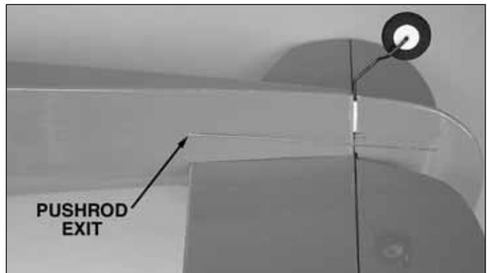
❑ 1. Insert the two wire pushrods into the outer pushrod tubes inside the fuselage. Notice at the aft end of the fuselage
